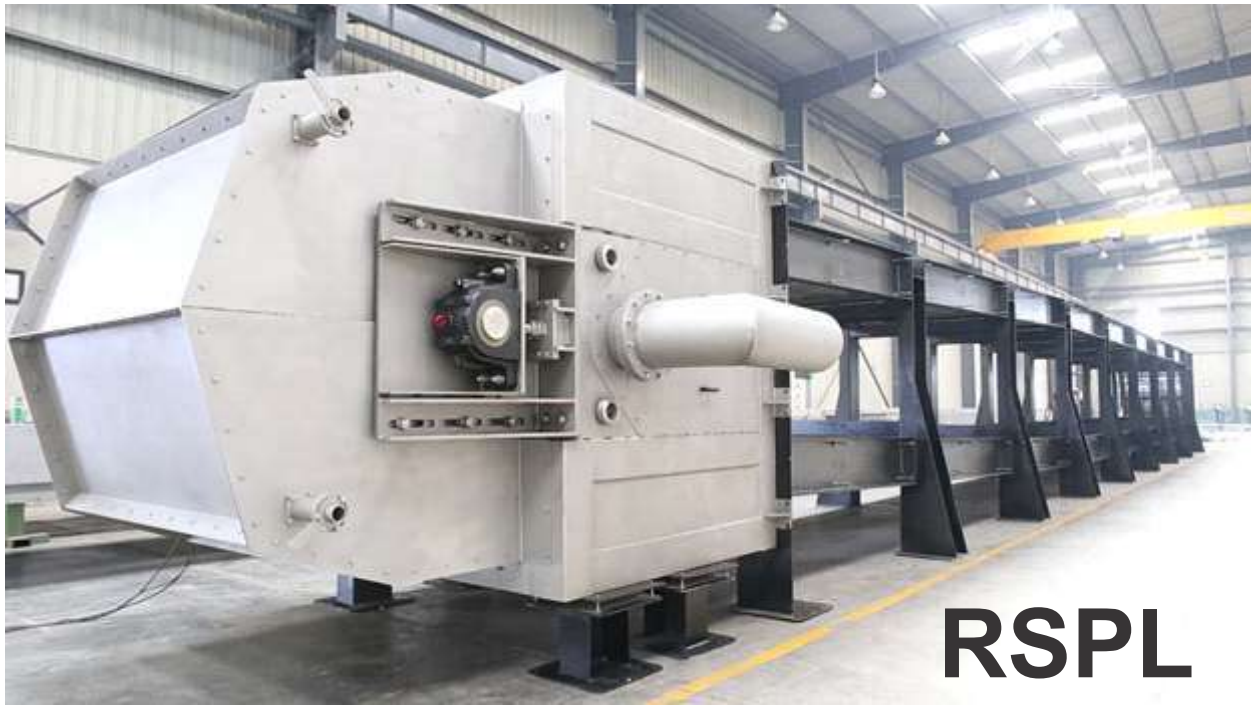
Complete Screen of over 31 meter length in Operational Testing at JASH for RSPL, Sea Water Intake, Dwarka, Gujarat (India)
