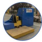
**Flight Forming Machine for** 5000 mm diameter
