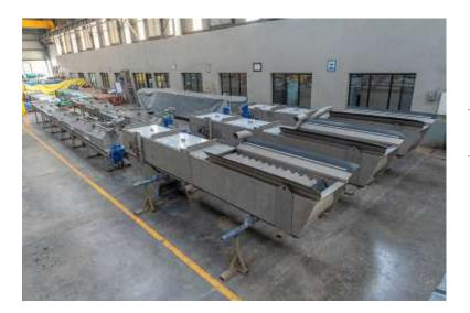
JMR Multirake Screens + Perscalator Screen + Screw Conveyor with wash Compactor & Automatic Deflection Plate Assembly
