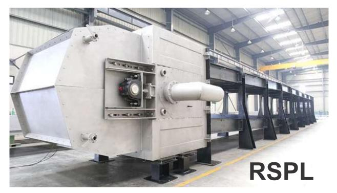
Complete Screen of over 31 meter length in Operational Testing at JASH for RSPL, Sea Water Intake, Dwarka, Gujarat (India)
