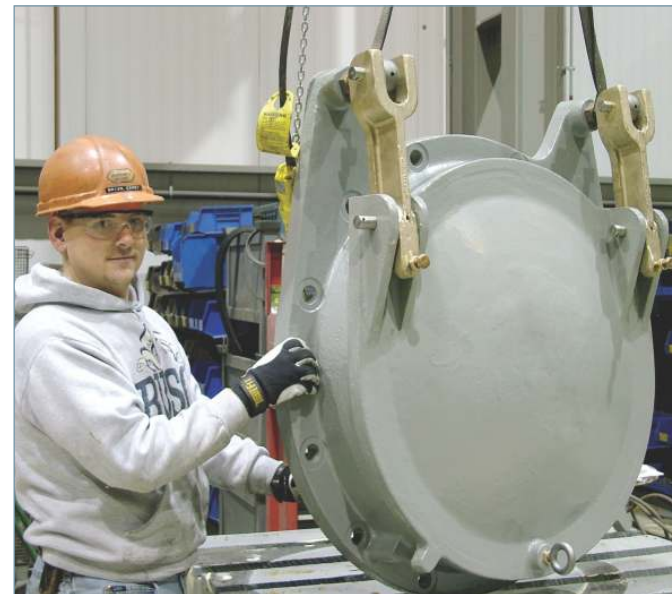
750 mm Diameter Flap Gates, 59th Ave Pump Station in Wickenburg, AZ, USA
