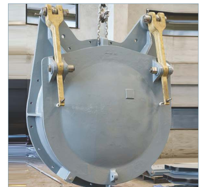
1800 mm Diameter Flap Gates, Russell Allison Ambraw Levee, Lawrenceville, IL, USA
