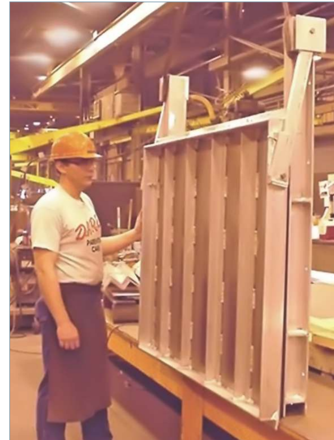
1200 x 900 mm Flap Gate, Metro Biosolids Center, San Diego, CA, USA
