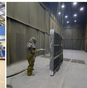
Shot Blasting Room (24 x 6 x 6m)
