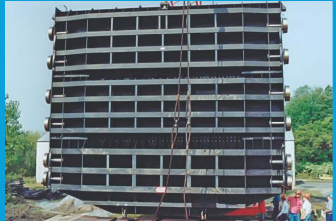
9000 x 8550 mm, Roller gate, Idaho Power's Swan Falls, ID, USA
