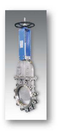
The MONO-T version Knife gate valve is bonneted, full lug, glandless valve in Cast Stainless Steel construction complying with AWWA C 520-10 and TAPPI standard. Mono-T version is having a single piece design up to DN150 and split body design above DN150.
