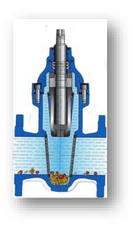
Sluice valves were developed for high pressure isolation application in water transmission lines. Sluice valve design incorporates two disc each having seating face corresponding to matching seat face on valve body. The disc are assembled in V shape groove provided in body. This two disc design enables a sluice valve to suit bi-directional application as well as offer very low leakage even in high pressure application.
