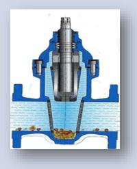
This valve can be provided with replaceable resilient seal encased in a replaceable seal retainer ring. Provision of this type of sealing avoids wearing of valve housing due to erosion and also enables easy replacement of seal at minimum cost and with low skill upon its wear.
