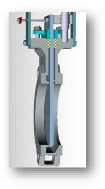
Knife gate valves were developed for isolation of pulp in paper industry where water contains large amount of solids in form of fibrous pulp. The gate of this valve was given a narrow edge at its bottom to enables it cut through settled pulp and achieve full closure of valve.
