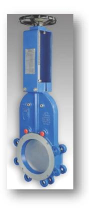
The MONO-A version Knife gate valves are bonneted, full Lug, gland less valve in Ductile Iron construction complying with AWWA C 520-10 standard. Full lug design enable end of line mounting without the need of additional flange. Mono-A version is having a single piece design up to DN 600 and split body design for higher sized valves.
