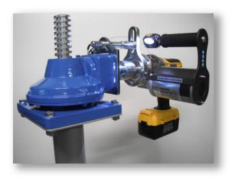
Portable battery driven actuators are provided to operate the gates in event of power failure for electric operated gates.
