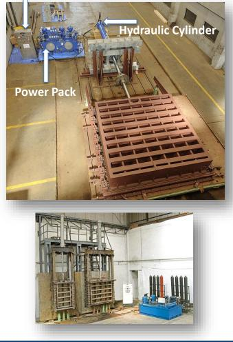
Hydraulic operation of sluice gate is recommended when faster closing of the gate in emergency is required or where fail safe condition is required.
