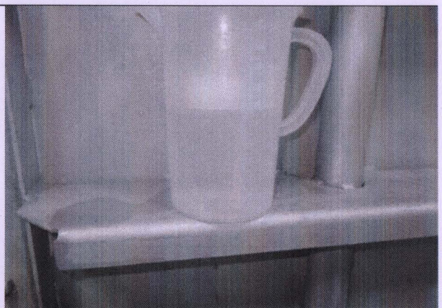
Description: Observed leakage rate before start operation cycle (Found 600ml).
