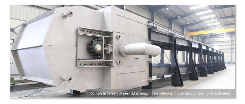
Due to large 31 meters length of screen, transportation of screens in assembled condition was not possible. Hence the entire 31 meter long structure was to be shipped disassembled and then reassembled vertically at site from bottom to the top. To assemble and hold the screens vertically at the same time was an installation challenge.
