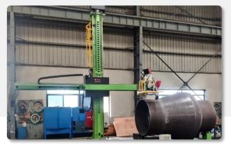
SAW Welding on Diameter upto 5000 mm
