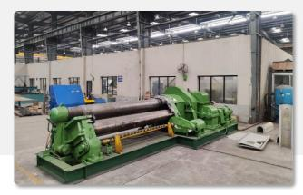
Roll Plates of 3000 mm Width & 30 mm Thickness.
