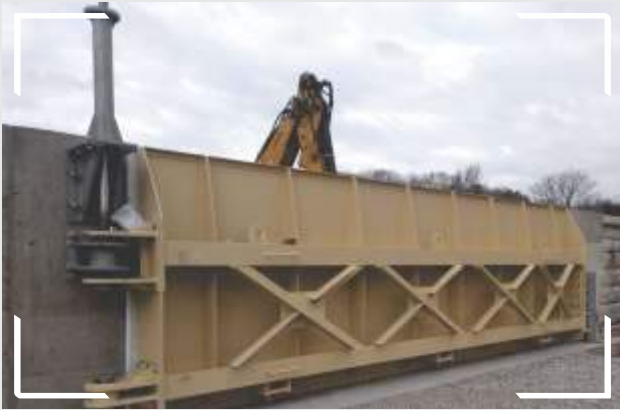
IAAW Davenport UV Disinfection Project, IA, USA Structural Steel Swing Gate 20'-8" X 9'-4 3/4" - 1 nos.
