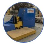
Flight Forming Machine for 5000 mm diameter
