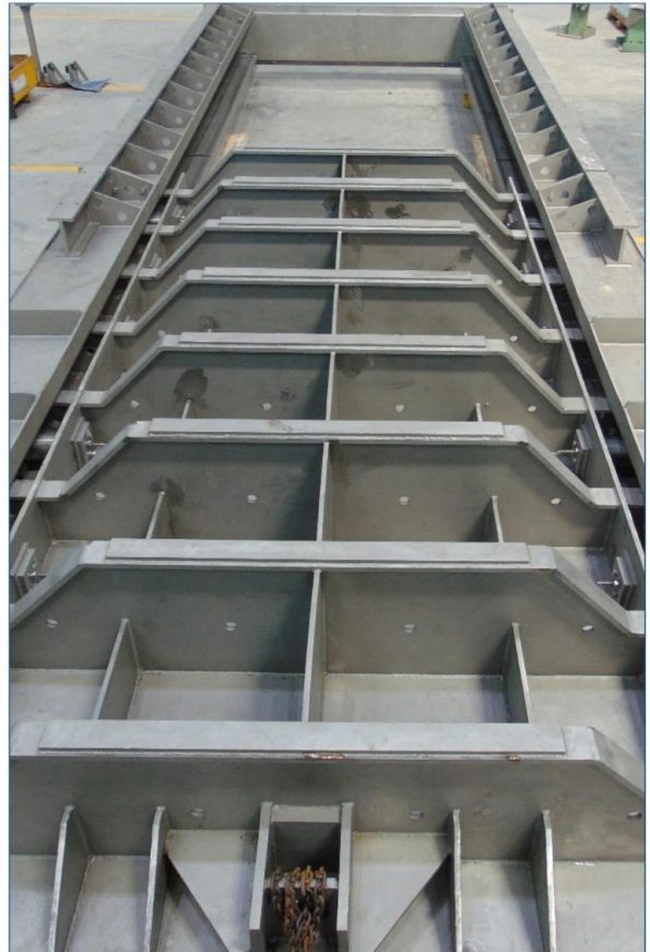
94.5" x 191" Stainless steel roller gate for C834 Doha South Terminal Pumping Station and Regional Odor control, Qatar
