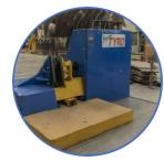
**Flight Forming Machine for** 5000 mm diameter
