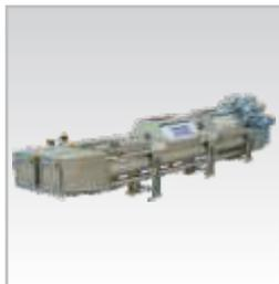
Screw Conveyor With Wash Compactor
